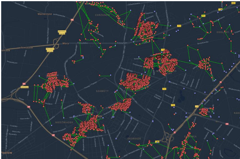
Fig. 5. Example fiber connections in the shortest distance model (green lines). Points marked red indicate locations in the list of white spots, blue dots indicate the location of the BTS. The area covered includes the Konotopa highway junction in Warsaw.
