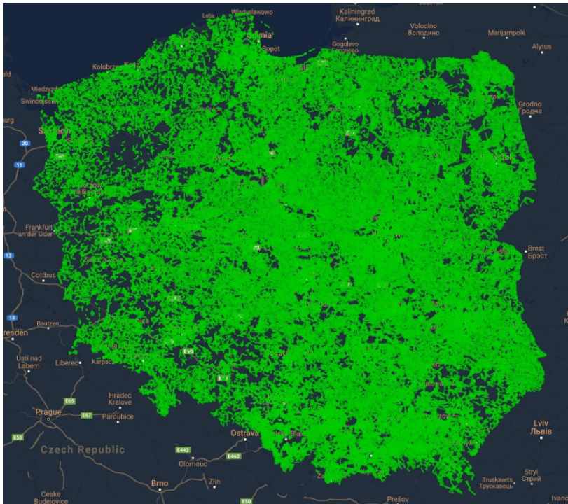
Fig. 7. Proposed path of optical fibers in the model of the shortest connections in the Polish scale. The total length of the connections required to connect all points from the list of white spots is 650,000 km.
