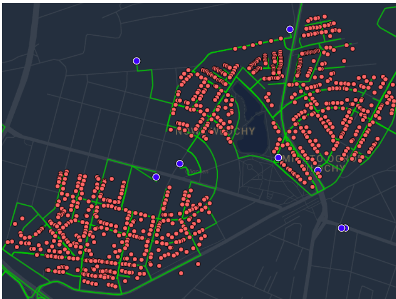
Fig. 6. Examples of fiber optic connections in a model where connections (green lines) are routed along roads. Points marked red indicate locations in the list of white spots, blue dots indicate the location of the BTS. The area covered includes Włochy (Warsaw).
